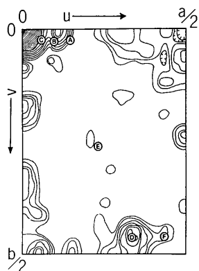
Fig. 3. Harker section (u, v, 0) of the three-dimensional difference Patterson synthesis of the Con-A \text{Hg}(\text{AcO})_2 derivative calculated to 5 Å resolution. Coefficients used are (\Delta F)^2 where \Delta F is as defined in the text. Letters indicate the expected Harker-section vectors for the sites listed in Table 1.
